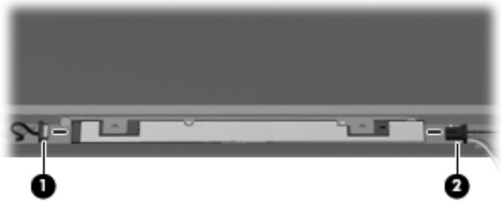
Disconnecting the Display Panel Cables
