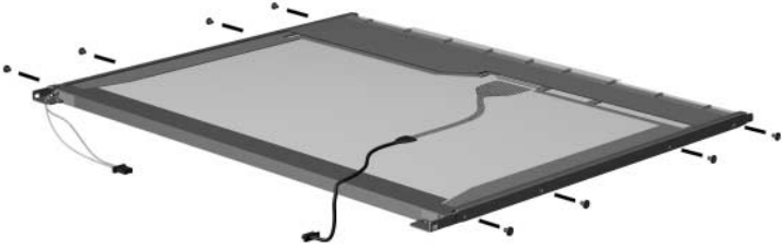
Removing the LCD Panel Frame Screws
